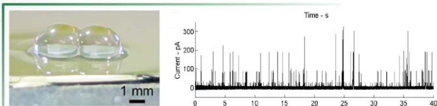
An air-stable droplet interface bilayer can be formed between non-coalescing water droplets on an oil-infused nanostructured surface.
