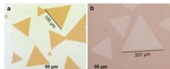
Optical micrographs of  $\text{MoSe}_2$  on  $\text{SiO}_2/\text{Si}$  and fused quartz
