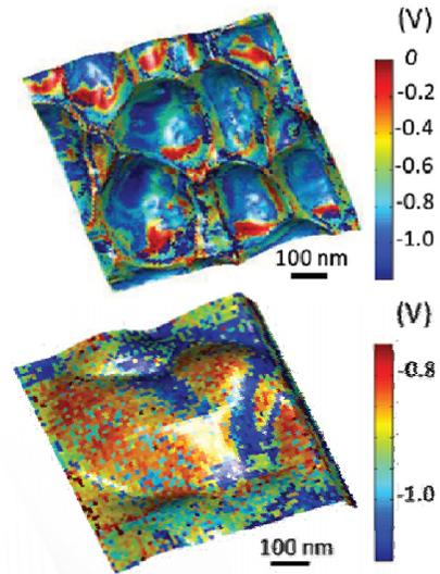
Surface charge overlaid on topographic image of undoped (top) and PCBM-infiltrated (bottom) perovskite film
