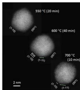
Tracking a single  $\text{Pt}_3\text{Co}$  at high temperature
