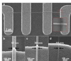
IBID benefits from smaller minimum probe diameter and beam penetration
