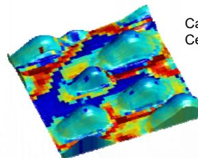
Catalyst Particles (Pt) on Fuel Cell Electrolyte Surface (YSZ)
